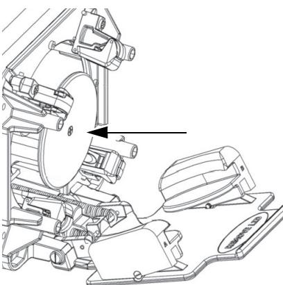
Use the Phillip's head screwdriver to loosen the remove the old lid plate.
