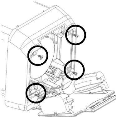
Use the Phillip's screwdriver to remove the housing screws
