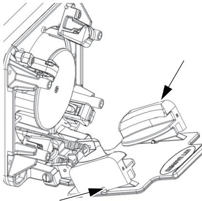
Using the standard screwdriver, loosen the claw screws and remove the current right and left side claws from inside the door.
