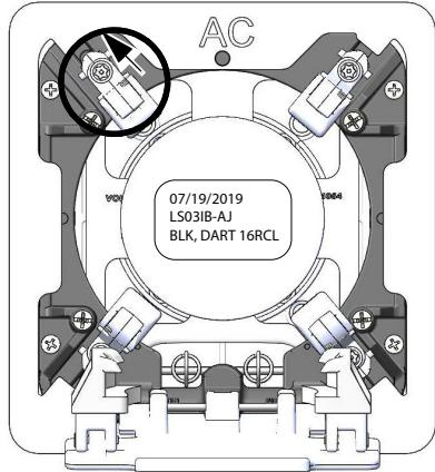
Place the pager template onto the flange with the tabs in the four pager slots. The template code must be facing up and outward.
