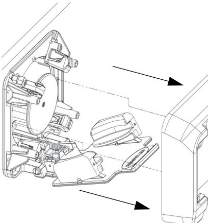
Remove the housing by pulling forward and allowing the housing to flex around the side edges of the open door.
