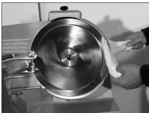
Figure 9. Cleaning the Ring Guard
