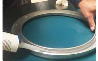
4. Turn the ring right side up and press it onto the rim of the drop-in until it is firmly seated.
